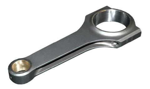
They are supplied ready balanced and equipped with our RMPi4 - 1552 bolts. These are UK manufactured with a UTS > 185,000 psi, and have resulted in the reliable operation using our RMPI4-1500 pistons to speeds in excess of 10,000 rpm.
