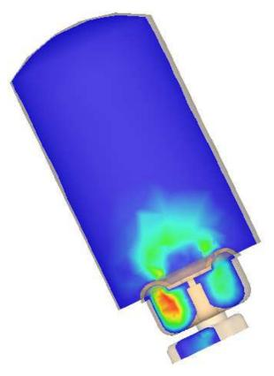
After the CAD model is finalised, an STL prototype is produced and tested on an engine running at 9500 rpm on our fully data equipped Dynamometer. The results are then compared to the initial design analysis. From this the final item is produced as a lightweight alloy casting and CNC machined for continual accuracy.
